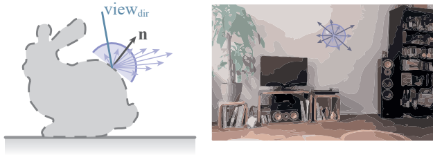
Fig. 6. Integrating the incoming radiance on a virtual object for rendering (left) and on a real surface for material estimation (right).
