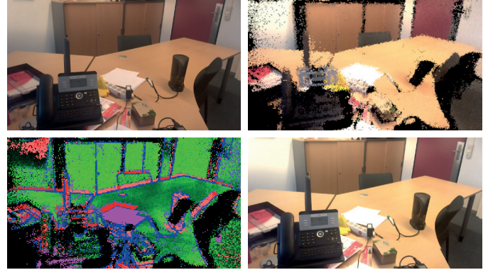
Fig. 3. Color Compensation. Top left : A camera input image in an unknown color space. Top right : The corresponding reference image rendered from the point cloud (see Sec. 6.1). Bottom left : The color-coded selection of sample pairs (green = valid). Bottom right : The corrected input image in the reference color space. Note that this process can output HDR values outside the [0, 1] range.
